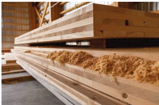
5-ply CLT (left) and SCL CLT
