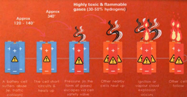
Thermal runaway can occur very quickly.
